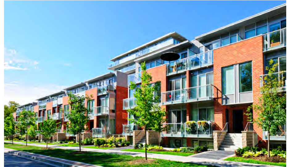
Grade-level entrances provide interest towards the street, while having a raised entrance to maintain privacy to the residential unit.
