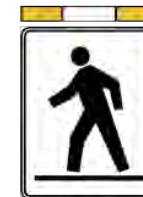
RRFB with RA-4 Signage
